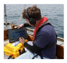
The PAM-Go electronics are housed in a robust case (IP67). A WiFi network is created to link the PAM-Go to a ruggedised tablet or laptop computer. Underwater sound is displayed and recordings made on the computer using the open-source software 'PAMGuard'. Hydrophone audio is streamed via cabled or Bluetooth headphones.
