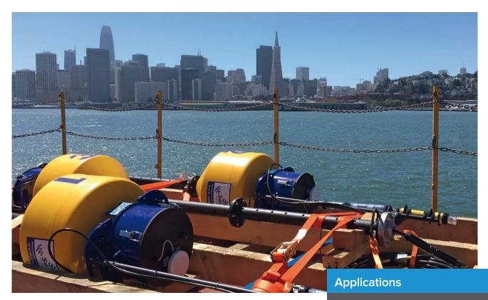
The system consists of a remote moored buoy with a multi-element detachable hydrophone array suitable for mitigation and anthropological noise capture. Signals can be captured up to a sampling rate of 500 ks/s at 16 bit depth. The system can be configured to record the data locally within the buoy or remotely at the receiving station, whichever is required.
