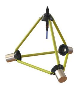
Employing a sensitive three-axis accelerometer, Hydraq QQ1000 can measure both orientation with respect to vertical, and hydrophone vibration (the latter typically caused by proximity to propulsion systems or Scholte waves at the water/seabed boundary). Vibration, typically a low frequency effect, can contaminate acoustic measurement and should be measured and accounted for.
