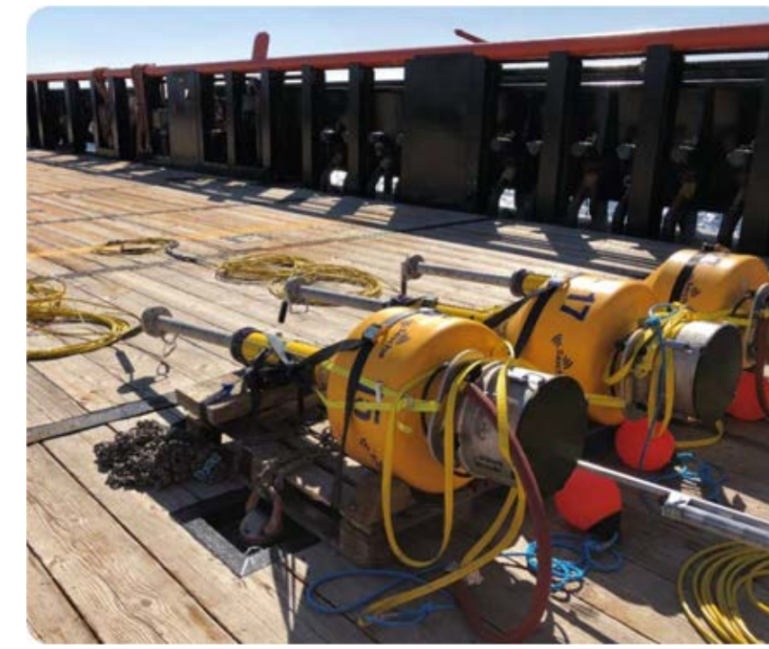
Figure 2 Drift buoys on board the survey vessel, before deployment.
