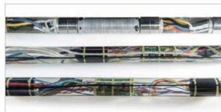
The Seiche Digital Thin Line Array is a high-performance, miniaturised underwater acoustic measurement device for static and low-speed towed monitoring applications.
