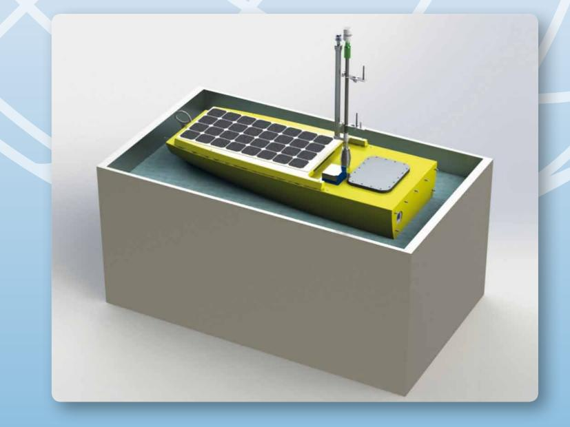
The hazard of floating ice to an unmanned surface vessel will be very real. AutoNaut has a well developed collision avoidance system based on marine traffic but requires development to enable work amongst floating ice. Enhanced situational awareness specifically for ice, such as thermal imaging, in concert with machine learning, will be developed for autonomous decisions on ice avoidance.
