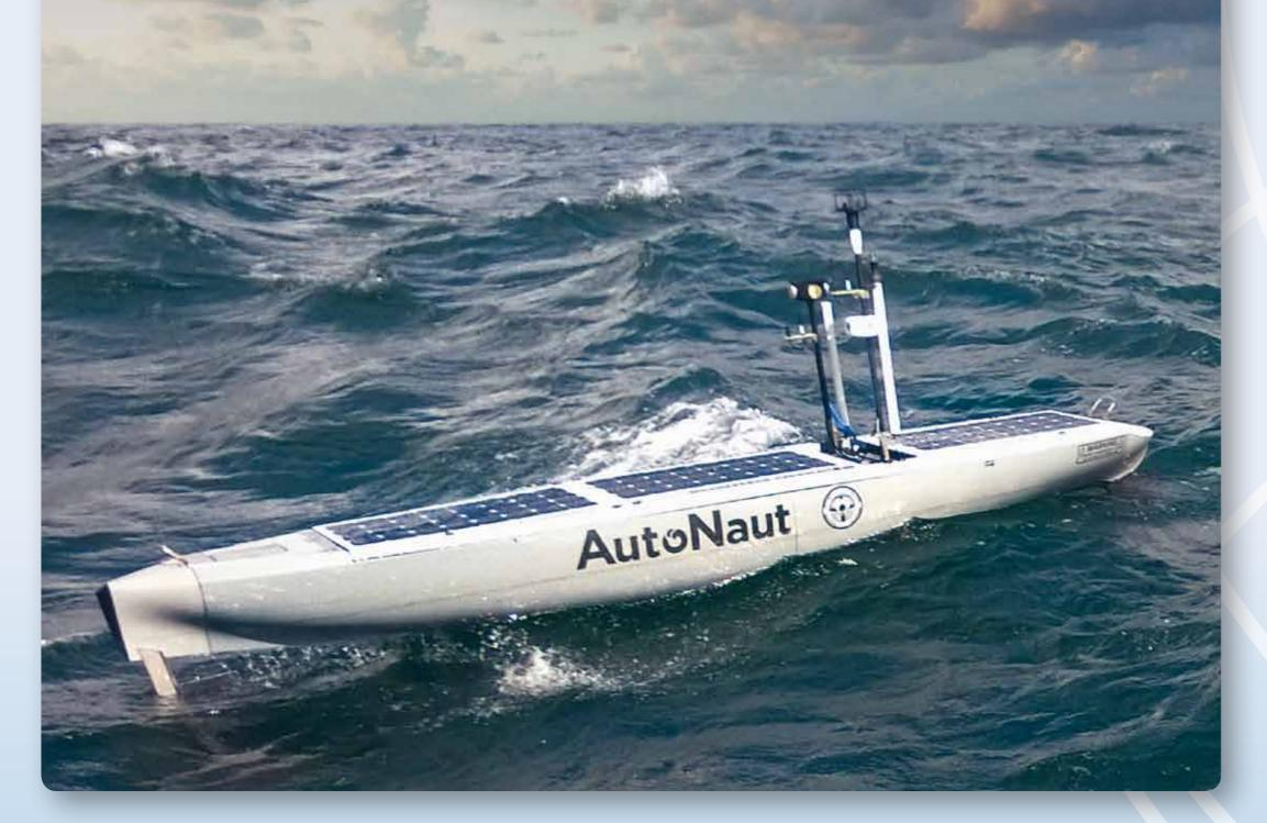
The AutoNaut is a wave propelled Unmanned Surface Vessel (USV) creating a step forward in autonomous data gathering. She has zero emissions, and can roam the oceans for very long periods, transmitting data via satellite to shore. With no requirement for offshore personnel, the AutoNaut significantly reduces costs and safety risks at sea. An extensive range of sensors and equipment can be installed.
