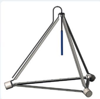
wireless link can also be provided from the onshore point of receipt to a listening station up to 2km away in line of sight. Installation is conducted by divers who secure the frame to the seabed using concrete blocks. SMART System requires specialist Seiche technicians in set up stage.
