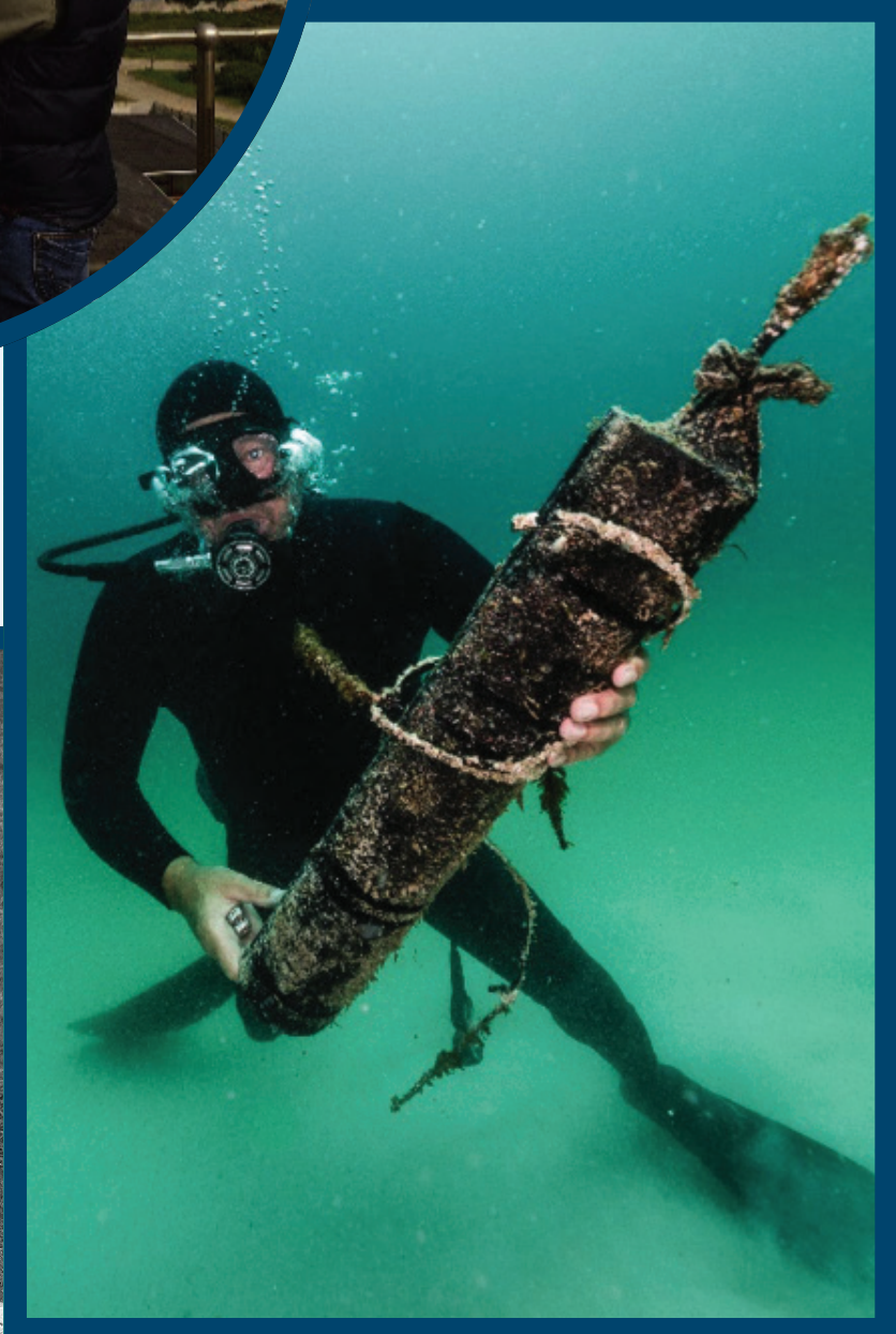
FIGURE 3 Diver retrieving the DSG-Ocean Loggerhead for a service and the custom designed mooring.
