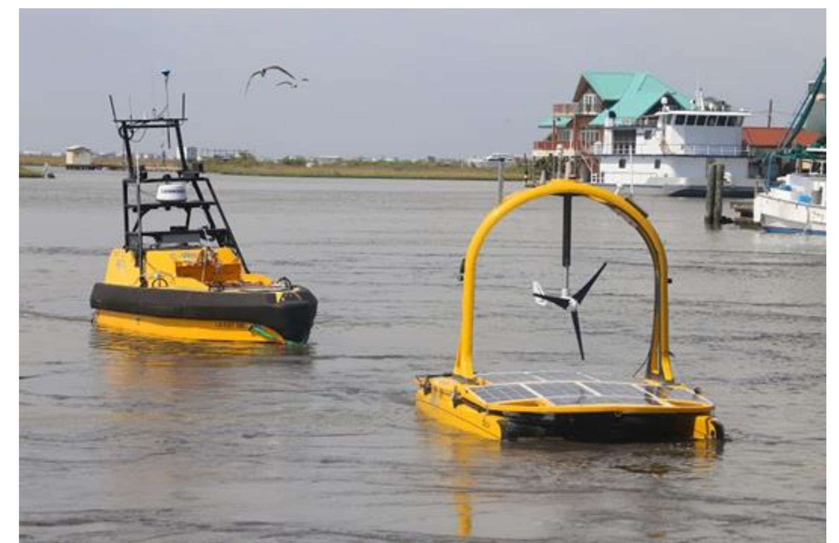
C-Enduro is a 4.2 m catamaran powered using a combination of solar panels, wind turbine and diesel generator, with two electric engines. It has a cruising speed of 3 kt and was designed for deployments of up to 90 day duration. C-Enduro towed a 55 m tow cable, with a single hydrophone.
