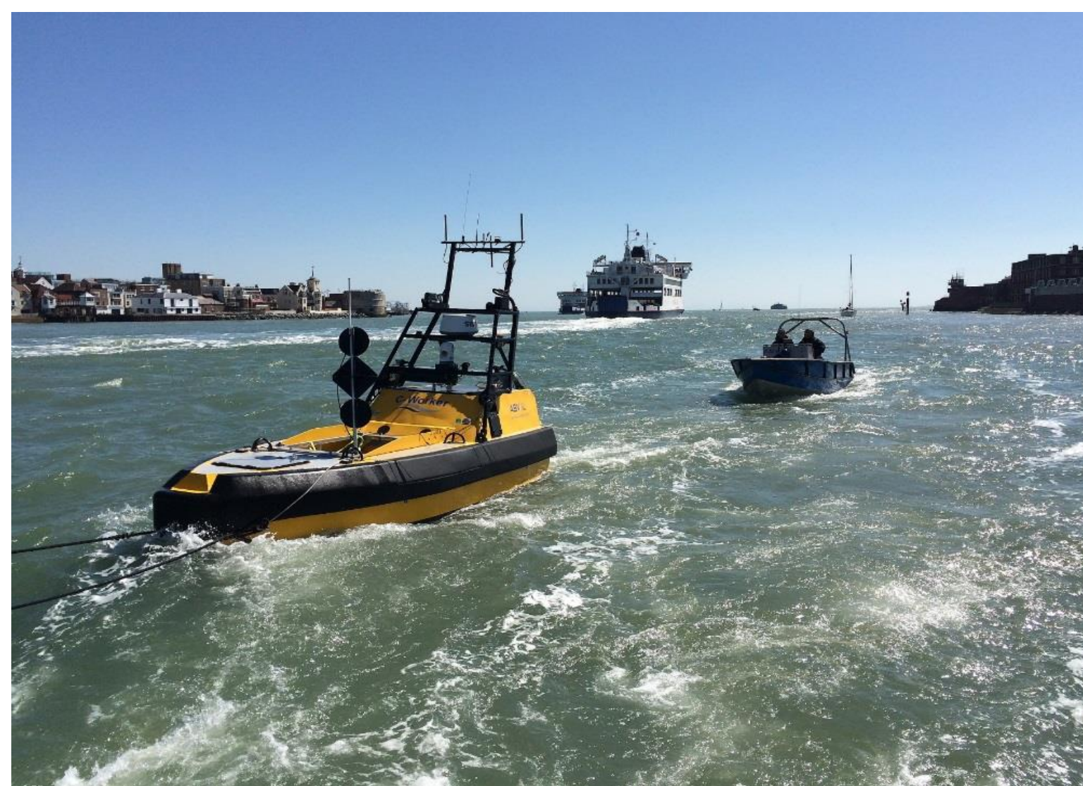
C-Worker is a 5.6 m long ASV. It has a displacement of 4.5 t, diesel-electric propulsion, twin propellers and a top speed of 6 kt. C-Worker deployed a 220 m tow cable with an array of two hydrophones and a depth sensor and an external CTD sensor-recorder.
