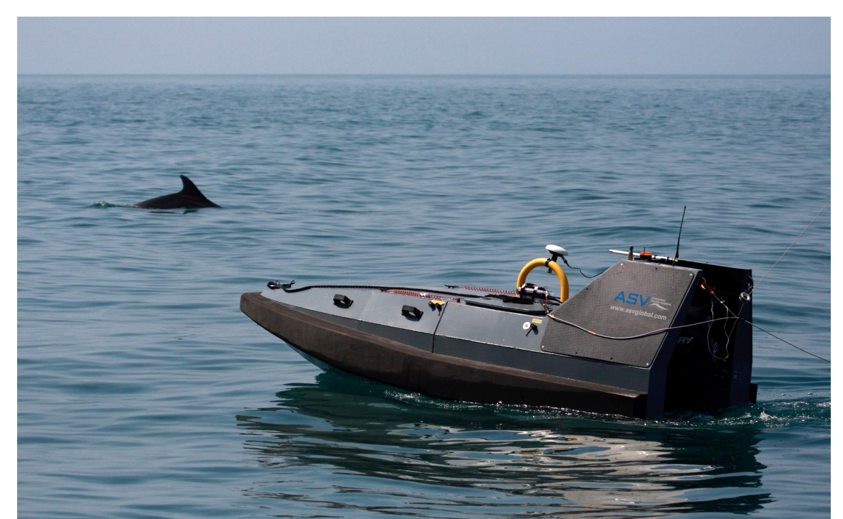
A 4 m ASV recording bottlenose dolphins with a towed hydrophone array during previous deployment trials in Cardigan Bay, U.K.
